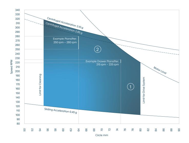
SIFTO's versatility is exemplified by its wide range of speed/throw combinations, facilitated by a large circle from approximately 55 mm to 80 mm and accelerations up to 3.1g:
