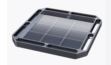
The screens sit low inside the tray, providing ample space for the product. This design not only maximizes capacity, but also seals against the outside without the need for felt or other gasket materials. A wide cross-section for throughs supports product flow, and the all-stainless-steel construction minimizes abrasion.
