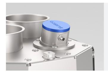
Utilizing SWISCA's proprietary radar probe, fill levels are measured without physical contact, ensuring robust and continuous operation - regardless of product processed.
