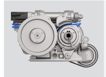
The bearings can be easily lubricated from outside the machine, allowing for maintenance without interrupting production. Integrated into the roll assembly, the lubrication system does not require removal for roll changes.
